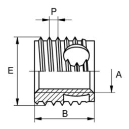
Female thread A = M10 Length B = 18 Male thread E = 14.0 Min hole depth blind hole = 22 Thread pitch P = 1.50
